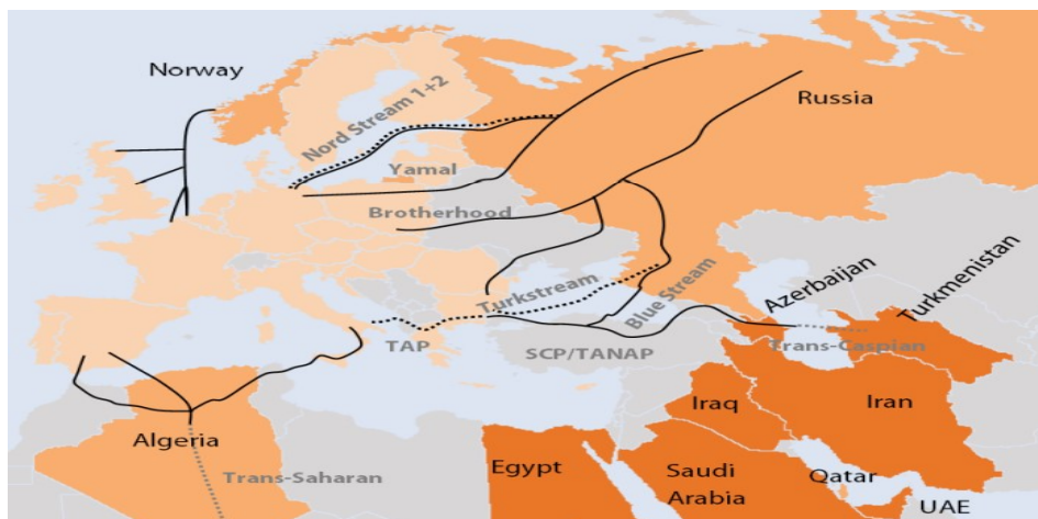
Fig. 1. The main external natural gas import pipelines of the EU (source: Energy security in the EU's external policy, 2020 )
