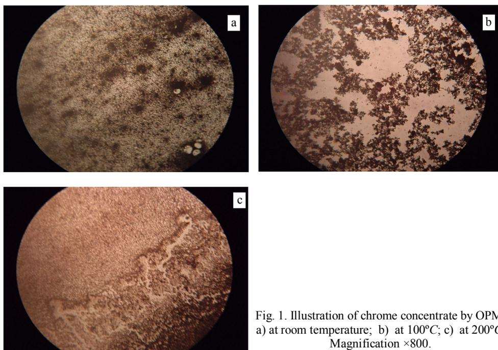
Fig. 1. Illustration of chrome concentrate by OPM: a) at room temperature; b) at 100°C; c) at 200°C. Magnification  $\times 800$ .
