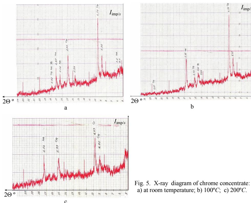
Fig. 5. X-ray diagram of chrome concentrate: a) at room temperature; b) 100°C; c) 200°C.
