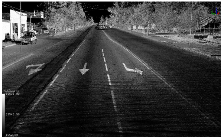
Fig. 1. Georeferenced point cloud obtained from scanning.
