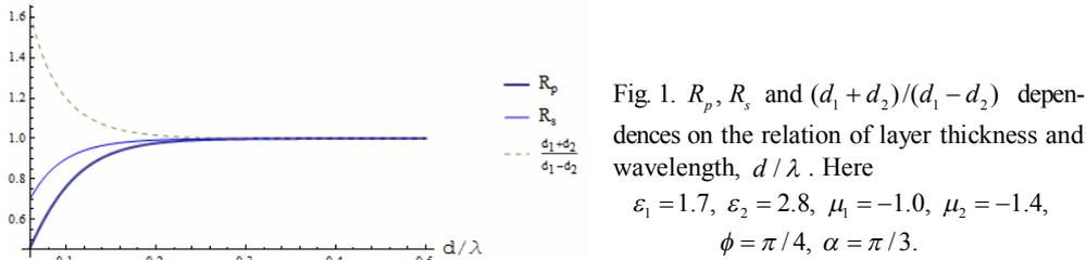
From those dependences one can see that the slight changes of optical axes orientation for fixed incident angle cause to the sharp variation of reflection coefficient, and opposite, for the fixed orientation of optical axis a small change of incident angle can lead to the big increase or decrease of reflection. All the characteristic parameters which bring different types of dispersion surfaces are taken from the analogical reflection coefficient studies of article [26].
