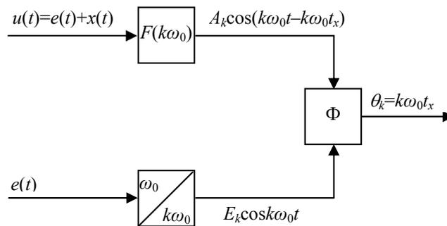
Fig. 2. The circuit for the measurement of the moment of perturbation on the  $k$ -th harmonic.
