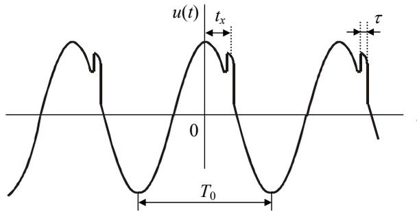
Fig. 1. Periodic perturbation of a harmonic signal.
