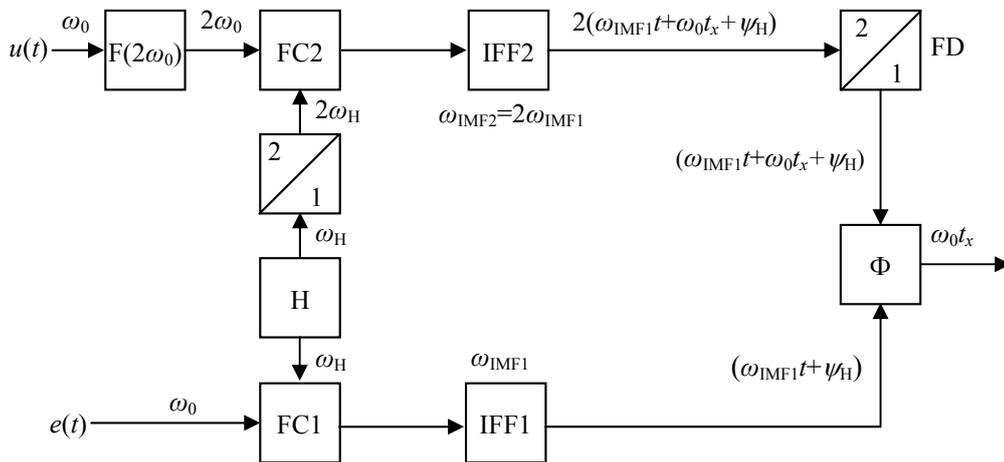
Fig. 3. The block-diagram of the device with expanded limits of the single-valued definition of the moment of perturbation.  $F(2\omega_0)$  – frequency filter, FC – frequency converter, IFF – intermediate frequency filter, H – heterodyne oscillator, FD – frequency divider,  $\Phi$  – phasemeter.
