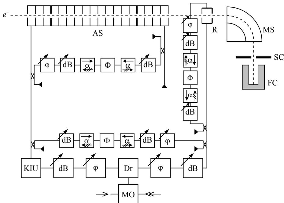
Fig. 4. Experimental layout. AS – accelerating section, R – RF-resonator, Dr – RF-preamplifier, KIU – 20 MW S-band klystron, MS – magnet spectrometer, SC – slit collimator, FC – Faraday cup.
