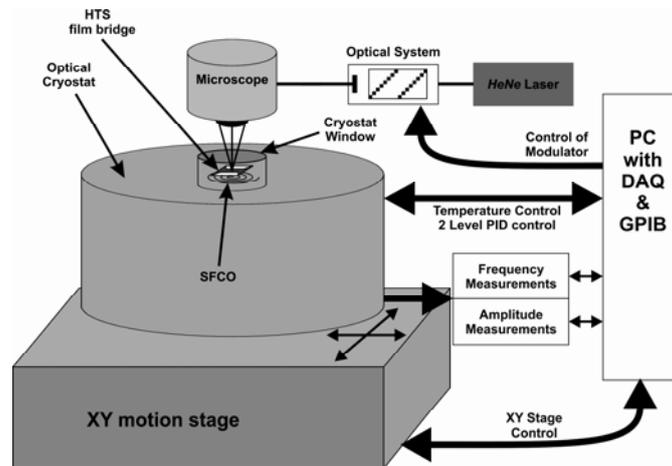
Fig. 2. Schematics of the SFCO-method based imaging technique, which uses a focused *He-Ne* laser beam as a probing signal.
