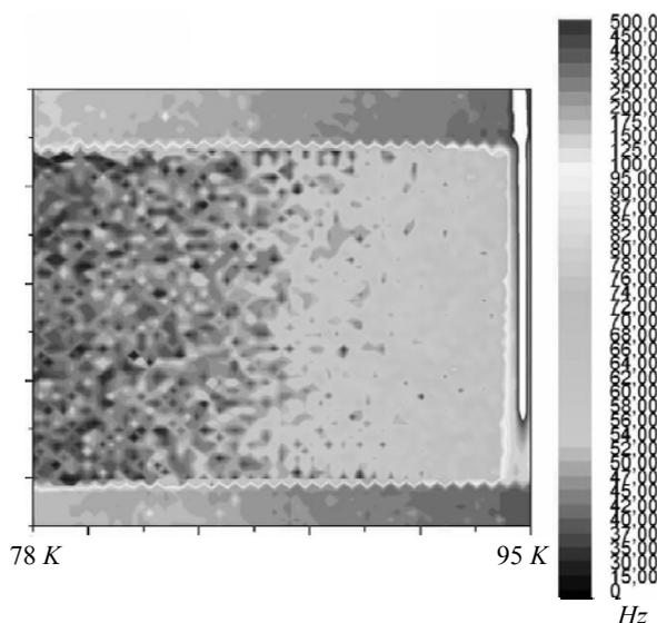
Fig. 4. 2D-imaging (visualization) of a phase transition of the tested YBaCuO composition HTS thin film bridge (200 μ wide) from the superconductive ( $T\sim 78\text{ K}$ ) to normal ( $T\sim 95\text{ K}$ ) state.
