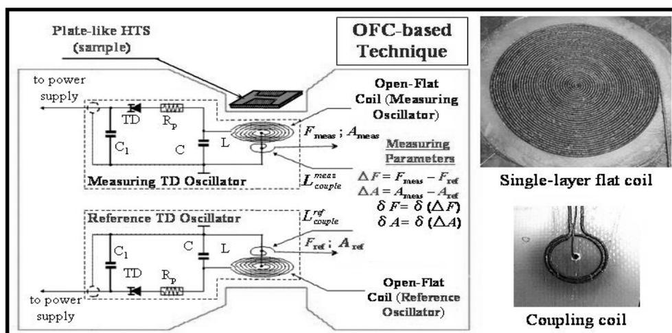
Fig. 1. Schematics of a single-layer flat-coil-oscillator based test-method, serving a basis for our imaging technique. Insets: the circular-shaped pick-up coil ( $\varnothing_{\text{coil}} \sim 3 \text{ mm}$ ) and the coupling coil.
