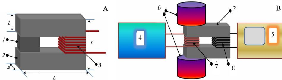
Fig. 2. A. YIG sample with magnetic sensor.
