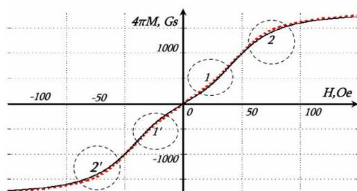
Fig. 3. Magnetization curve for the monocrystalline YIG sample with the ferrite sensor: dot line – experiment; solid line – approximation.
