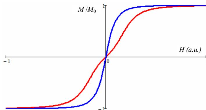
Fig. 1. Typical forms of magnetization curve of soft ferromagnetic materials.
