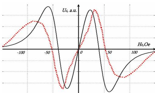
Fig. 4. Dependence of the detected signal magnitude on the external magnetic field: dot line – experiment; solid line – simulation result.
