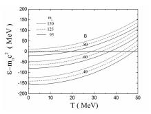
Fig. 2. Energy per baryon  $\varepsilon(n_0, T)$  for SQM at zero pressure as a function of temperature for different values of model parameters *B* and  $m_s$ .
