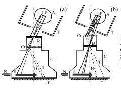
Fig. 1. Experiment diagram: T is X-ray tube; A is anode; LF is linear focus; C is chamber; Cr is studied crystal; D is diaphragm; S is immovable valve; F is photographic plate; N is permanent magnet; H is diffracted radiation.
