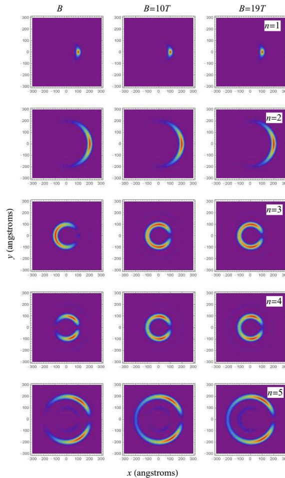
Fig. 3. Electronic probability densities in the five lowest states for different values of magnetic field induction when impurity is in the inner ring.
