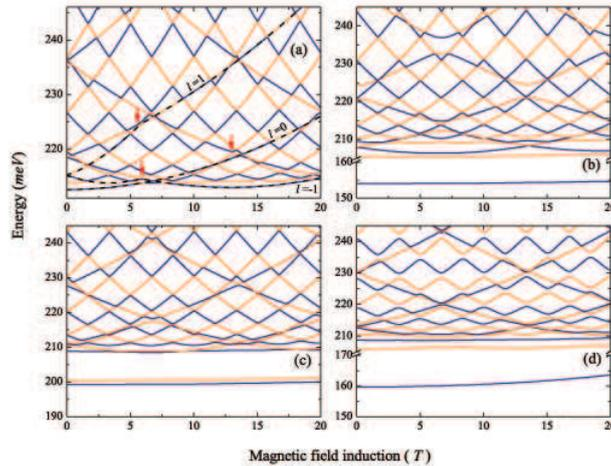
Fig. 2. Dependencies of electron energy on magnetic field induction in the absence of impurity (a), in the presence of an impurity positioned in the inner ring (b), in the presence of an impurity positioned in the barrier region between the rings (c) and in the presence of an impurity positioned in the outer ring (d). The red arrows indicate on the anticrossings, which are not the consequence of the symmetry breaking.
