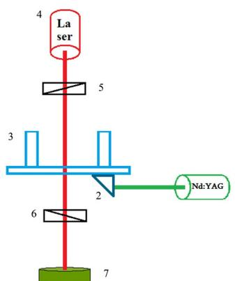
Fig. 1. Scheme of the experimental setup. 1 – Nd: YAG quasi-continuous laser; 2 – prism; 3 – cell; 4 – probe laser; 5, 6 – polarizers; 7 – power meter.
