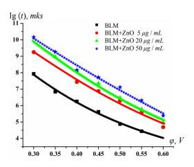
The decrease of the average lifetime of BLM at increasing potential in the presence of ZnO nanoparticles at given concentrations. Points are experimental data (average of 5 measurements at each potential difference) and solid lines are theoretical curves from least-square fitting using Eq. (2).
