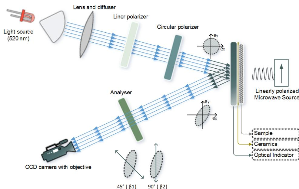
Fig. 1. Schematic diagram of the TEOIM.
