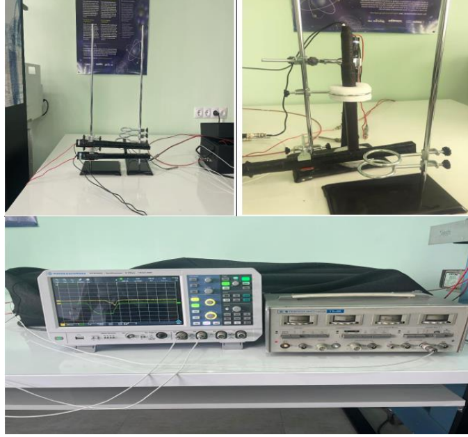
Fig. 6. The light yield (LY) is measured by the number of photoelectrons registered.
