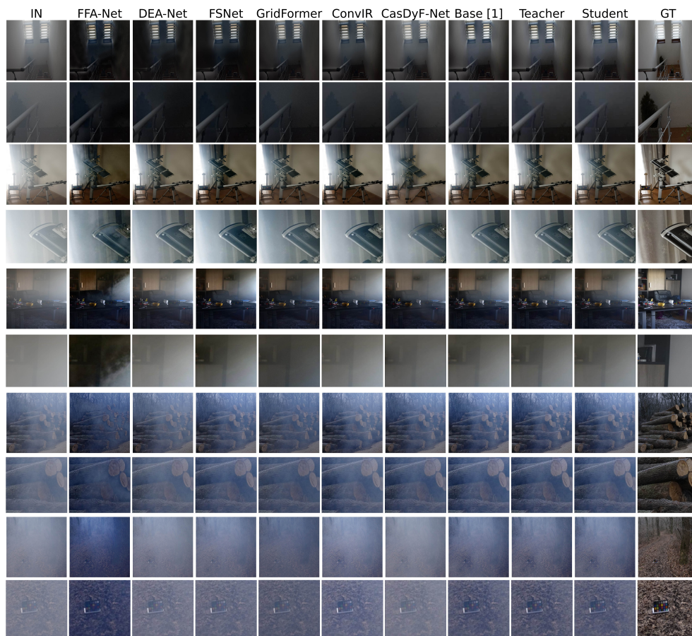
Qualitative comparison of dehazing results on real-world images from O-Haze and I-Haze datasets and Haze4k synthetic dataset. All competing methods have been trained on the synthetic Haze4k dataset. The IN and GT columns correspond to the observed and ground-truth images, respectively.
